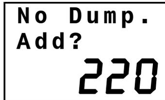
The operator can manually Accept (Add) the measured weight if valid. Refer to page 11 for more details on Adding weights.
